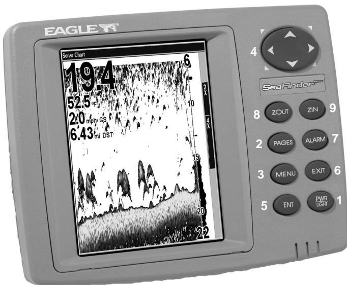
The SeaFinder 640c DF sonar unit showing full sonar chart screen display and keyboard.
